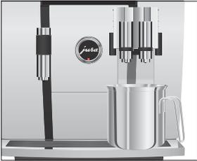
When you switch off your GIGA, the dual spout is rinsed automatically.
