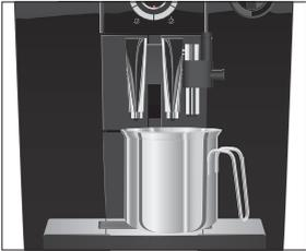
When the IMPRESSA is switched off, the system is automatically rinsed if a specialty coffee has been prepared. If cappuccino or milk foam has been prepared, the machine will also prompt you to rinse the cappuccino frother.
