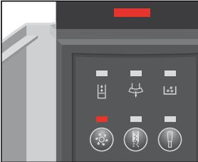
The illuminated maintenance indicator draws your attention to the maintenance actions that are necessary. Open the access door and note the further indicators in the maintenance field. In the example shown on the left, your IMPRESSA is prompting you to clean it.
